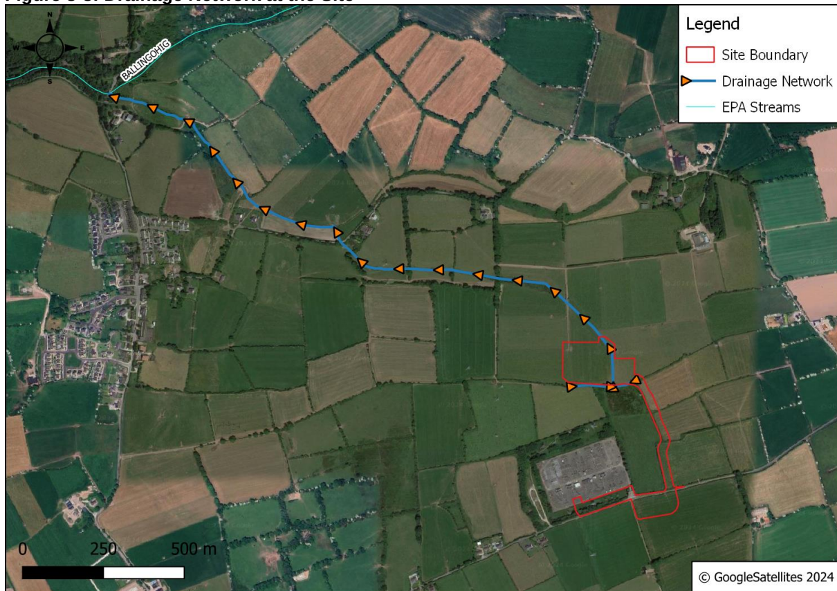
Figure 3-3: Drainage Network at the Site
